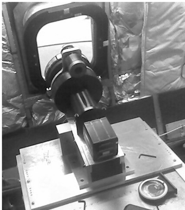
Fig. 1 IHFRI as mounted in NASA's DC-8 Airborne Laboratory. The top cylinder is the mount for a photomultiplier tube, and the bottom assembly shows the grating, lens, intensifier, and CCD camera, respectively.
